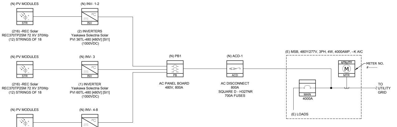
NOTE: PV SYSTEM OUTPUT CONDUCTORS TO BE CONNECTED PER NEC 690.64, 705.12, 240.21, 230.82, 312.6(A) & 312.6(B). EXISTING PANEL BUSSING WILL NOT REQUIRE MODIFICATION OR RE-CERTIFICATION OF THE SWITCHGEAR BY U.L. ALL CONNECTIONS WILL BE IN THE CUSTOMER SIDE OF THE GEAR AND WILL NOT REQUIRE REMOVAL OF BARRIERS OR ROUTING THROUGH UTILITY SECTIONS.
