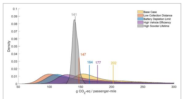
**Figure 3.** Shared e-scooter Monte Carlo analysis of global warming impact. Kernal density functions show the Base Case and four alternative collection and distribution scenarios: low collection distance, battery depletion limit, high vehicle efficiency, and high scooter lifetime. Colored vertical lines indicate the mean value for each scenario.
