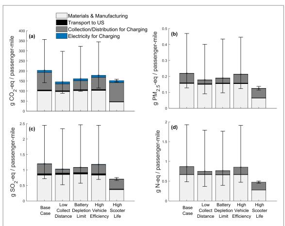
**Figure 2.** Life cycle environmental impacts for shared electric scooters under Base Case and alternative collection scenarios for (a) global warming, (b) respiratory effects, (c) acidification, and (d) eutrophication. Error bars represent 95% of the Monte Carlo simulations.
