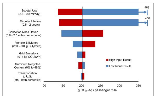
**Figure 4.** Sensitivity analysis of global warming potential for various shared e-scooter scenarios. This sensitivity uses the average value from the base case scenario as seen previously in figure 3, but applies a static low and high value to the input parameter of interest shown in parentheses along the y axis.
