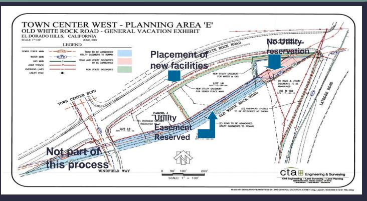
Site development plans have been submitted to the DOT, which identify the relocation of utility facilities to other areas parallel to the new realigned roadway.
