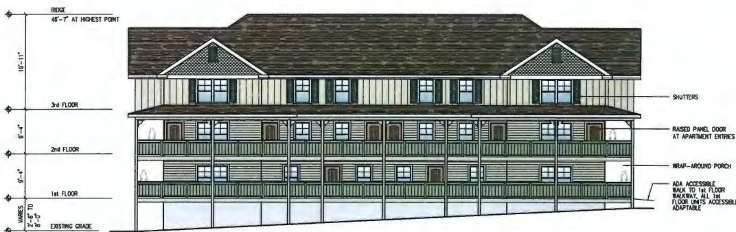
2 EXTERIOR ELEVATION - BUILDING B SOUTH (FRONT)
