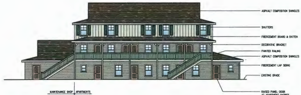
3 EXTERIOR ELEVATION - BUILDING C SOUTH (FRONT)
