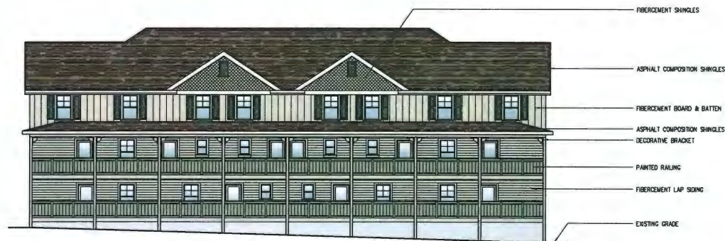
1 EXTERIOR ELEVATION - BUILDING B NORTH (REAR)
