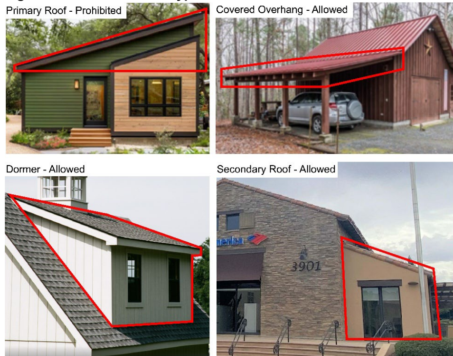
Figure 7 Shed Roof Types
