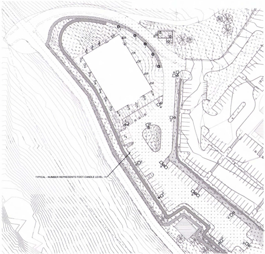
1 ENLARGED SITE PLAN - ELECTRICAL SCALE: 1" = 30'-0"
